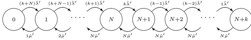
Since we are working with a memoryless model, we assume exponential distributions for both mill lifetimes and roll pair replacement times.<sup>5</sup> To calculate the cost function  $c(t)$  in terms of  $\hat{\mu}$  and  $\tilde{\lambda}$  for  $t \rightarrow \infty$ , we obtain the equilibrium distribution  $\pi$  by solving
